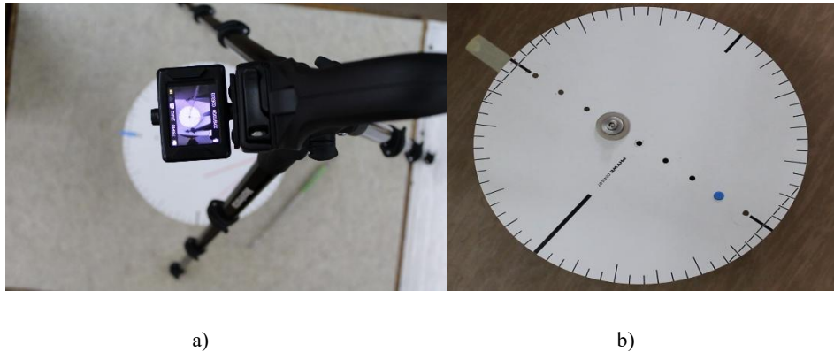
Fig. 6 – Experimental setup to measure the oscillation period of the disk. a) general view from above; b) detail with the disk having the oscillation center at the first hole situated at a = 3\text{cm} from the mass center of the disk. The full color version may be accessed at https://rrp.nipne.ro .
