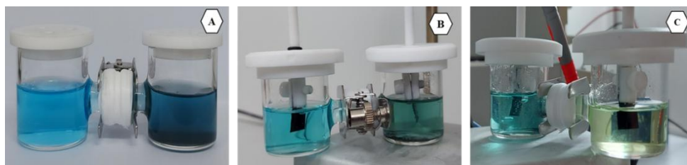
Fig. 8 – VRFB battery with V^{4+} - V_2C MXene electrolyte solution at a 1:9 dilution ratio (anolyte in right compartment), showing charging color stages: (A) initial blue V^{4+} anolyte and catholyte, (B) first visible V^{3+} reduction signs after 2 hours, and (C) final green V^{3+} anolyte and yellow V^{5+} catholyte after 24 hours. The full color version may be accessed at https://rrp.nipne.ro .
