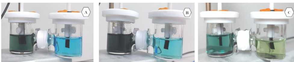
Fig. 11 – VRFB battery with \text{TiC}_2 -based Mxene at a 1:9 dilution ratio, showing color stages during charging: (A) initial blue \text{V}^{4+} anolyte and catholyte, (B) obscured color transition due to the magnetic stirrer and Mxene concentration, and (C) final green \text{V}^{3+} anolyte and yellow \text{V}^{5+} catholyte, confirming successful redox reactions. The full color version may be accessed at https://rrp.nipne.ro .
